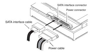
Figure 4. Attaching SATA cabling
